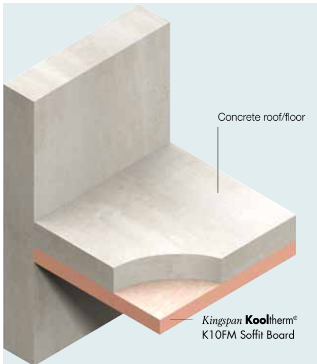
Figure 1 Concrete soffit floor installation
